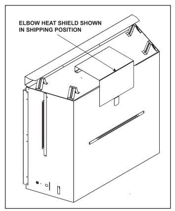
Figure 9.1 Elbow Shield Shown as Shipped
